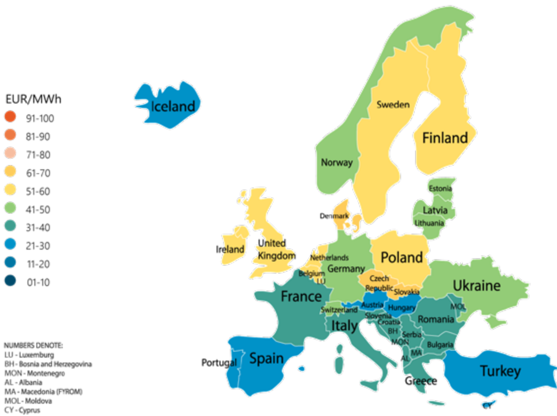
Fig. 21. Levelised cost of electricity across Europe in 2050 (Source: LUT University and Yélé Consulting, results of the moderate scenario)
