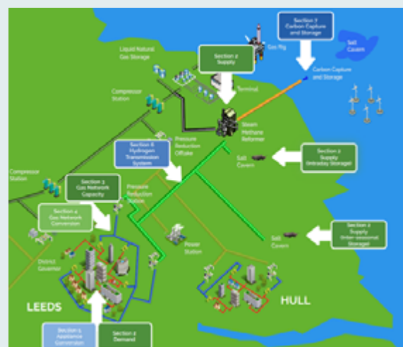
Fig. 11. H21 Leeds City Gate System Schematic (Source: H21 Leeds City Gate project, 2021)
