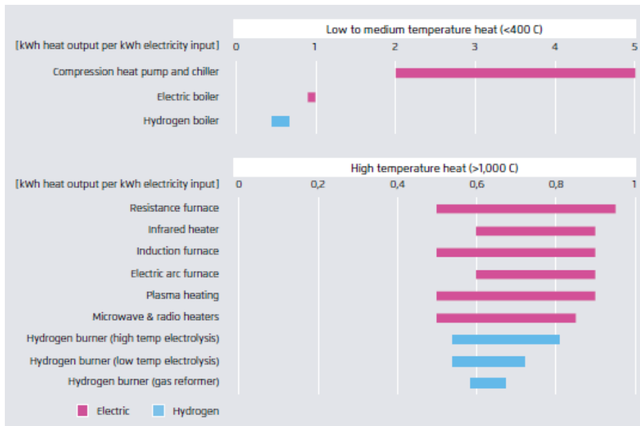
Figure 9 : Performance factors of power-to-heat technologies vs. heat from burning hydrogen derived from electrolysis (Agora Energiewende - Afry, 2021)
