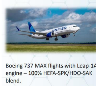
Boeing 737 MAX ground & flight tests with Leap-1B engine – 100% HEFA-SPK.
