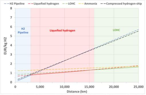
Figure 2 Hydrogen delivery costs for a simple (point to point) transport route, for  $1 \text{ Mt } H_2$  and low electricity cost scenario.
